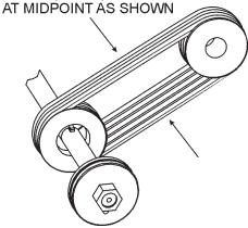
Figure 17. V-Belt Tension
